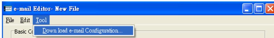
The "Email Configuration transfer" window will appear at this time; in the "Target IP" field, fill in the IP address of the FBs-CBEH expansion board to download the information, then confirm that the correct password is entered in the "Password" field and press the "Start Download" to perform the downloading.
