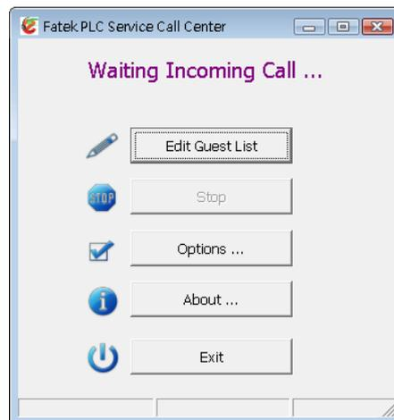
The Service Call Center software is provided to work with remote maintenance operations, used to perform maintenance tasks when the PLC workstation's IP is acquired with the dynamic IP method or when it is in a more complicated network environment and the IP is difficult to acquire. Please refer to Chapter 8 for detailed operation contents.
