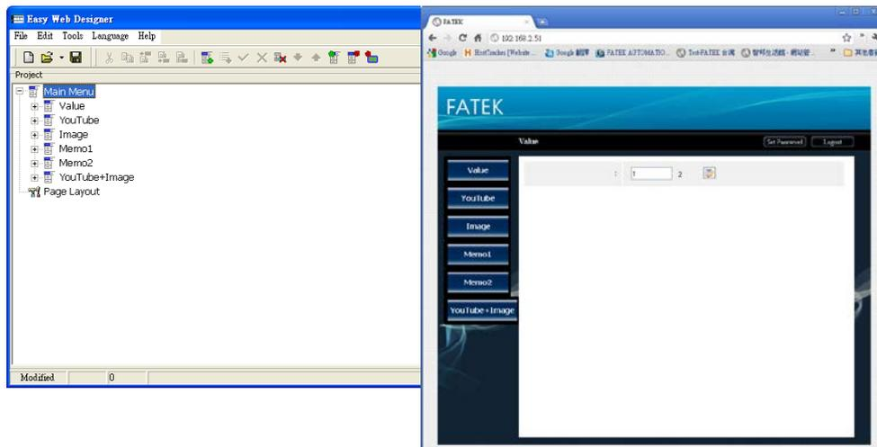
The FBS-CBEH expansion board provides the function to allow users to easily browse or control the status within the PLC through a customized web page; the customized web page can be created through this software without requiring the user to have the skills to write HTML. Please refer to chapter 4 for detailed explanation.
