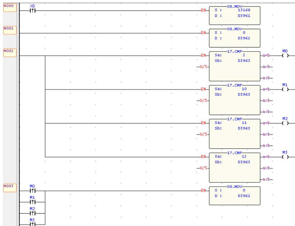
After completing the steps mentioned above, every time X0 changes from 0 to 1, and when D3962 is 0, the mobile phone will receive the SMS sent by the FBs-CBEH expansion board.
