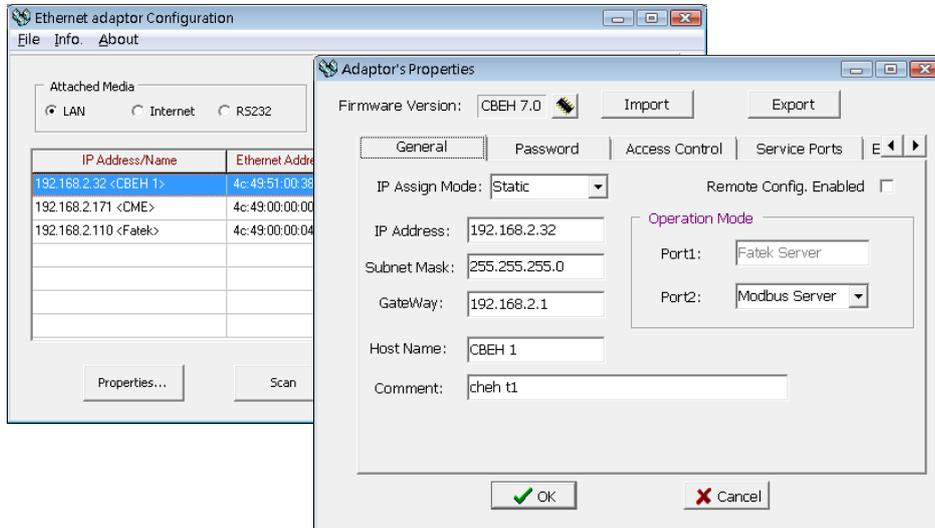
An application that works with the FBS-CBEH expansion board provides a window-based configuration software, used to set the module's basic settings, password protection and firmware update etc. Please refer to Chapter 3.1 for detailed explanation.
