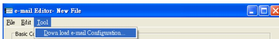
The "Email Configuration transfer" window will appear at this time; in the "Target IP" field, fill in the IP address of the FBs-CBEH expansion board to download the configuration, then confirm that the correct password is entered in the "Password" field and press the "Start Download" to perform the downloading.
