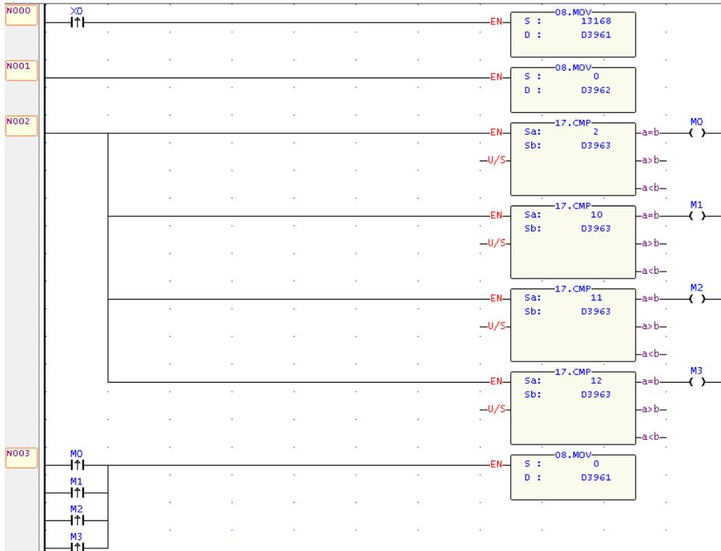
After completing the steps mentioned above, every time X0 changes from 0 to 1, and when D3962 is 0, it will receive the Email sent by the FBs-CBEH expansion board;
