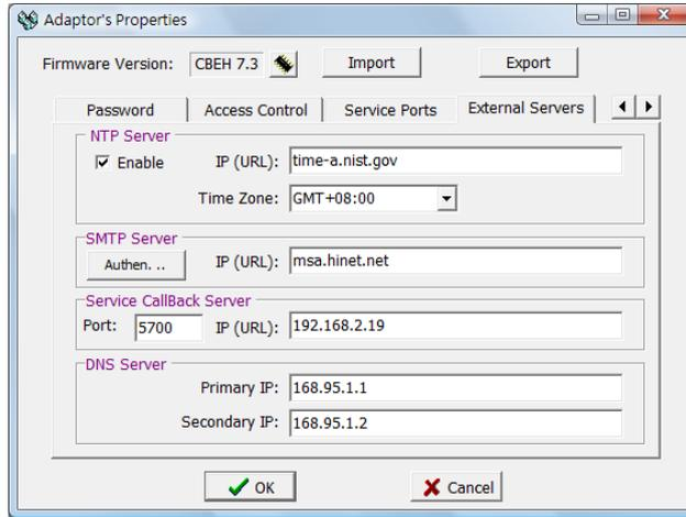
**NTP Server:** The CBEH expansion board provides the internet clock synchronization function, eliminating the trouble of manually correcting the time on a regular basis. To activate this service, just check Enable; when the service is activated, it will periodically request the newest clock data from the NTP server and set the data into Calendar register (D3953~D3960) accordingly (Please refer to Chapter 6 for details).
